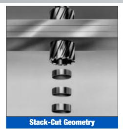
Rotabroach Annular Cutters with a Stack-Cut tooth geometry must be used whenever two or more plates are being drilled simultaneously. With our exclusive end tooth design, stacked materials can typically be drilled in a single pass.
